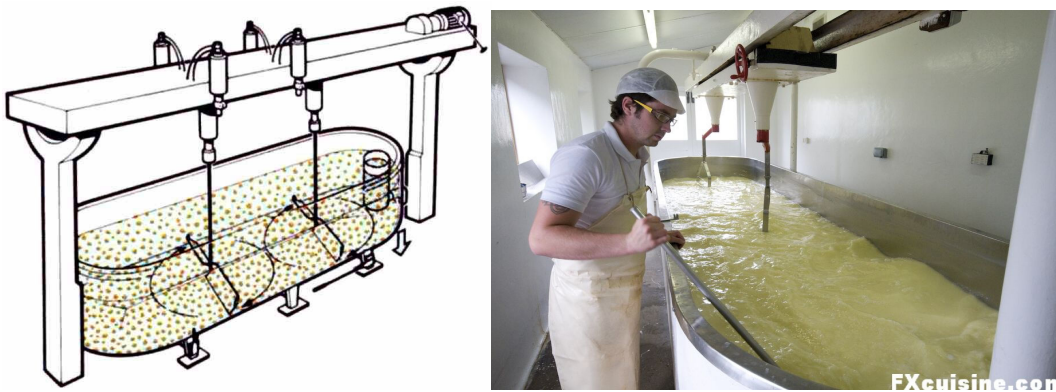
Figure 5. The drainage of whey from a traditional cheese vat by a perforated cylinder
