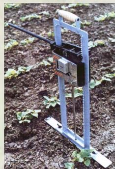
Figure 2. 3T System hand penetrometer
