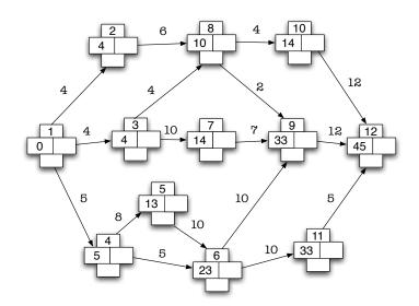
$$\begin{array}{rcl} T_{11}^1 &=& 45-5=40 \\ T_{10}^1 &=& 45-12=33 \\ T_9^1 &=& 45-12=33 \\ T_8^1 &=& \min\{33-2;33-4\}=29 \\ T_7^1 &=& 33-7=26 \\ T_6^1 &=& \min\{33-10;40-10\}=23 \\ T_5^1 &=& 23-10=13 \\ T_4^1 &=& \min\{13-8;23-5\}=5 \\ T_3^1 &=& \min\{26-10;29-4\}=16 \\ T_2^1 &=& 29-6=23 \\ T_1^1 &=& \min\{23-4;16-4;5-5\}=0 \end{array}$$
