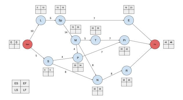
As a result, we can see that the length of the longest path is 46 (unit of time): that is the ES (and EF) numbers we obtained in the 'Fin' node.
