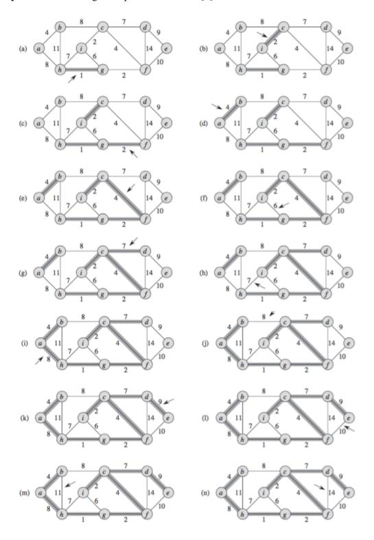
The small arrows on the figures show which edge is currently considered by the algorithm. The shaded edges belong to the spanning tree. Note that in many steps the algorithm merges separated trees, so during the execution we might obtain forests, but upon finishing we have the minimum spanning tree.
