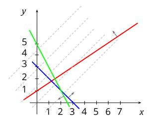
the possible solutions for the objective function are shown as gray dashed lines. We need to look for the one which crosses the feasible region and the y value is maximized. That is (4/3,7/3) for which we obtain 19/3.
