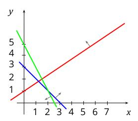
The red line corresponds to the father's constraint, the blue line for the mother's constraint, and the child's capacity is represented by the green line. Together with the x and y axes (so 5 lines altogether) they give the space of the feasible solutions.
